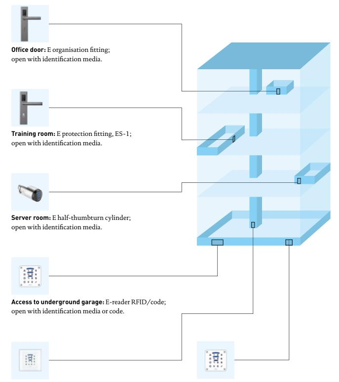
**Lift:** E-reader RFID/code with selective floor control; control with identification media or code.
