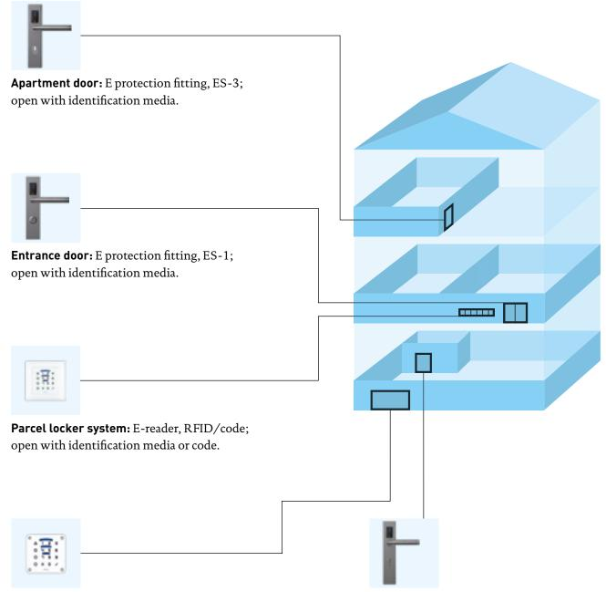
**Access to underground garage:** E-reader RFID/code; open with identification media or code.
