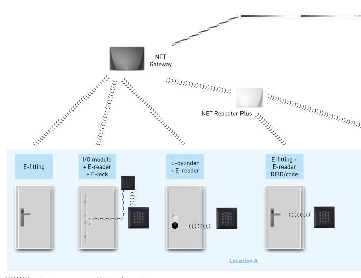
Transmission via LAN/WLAN (TCP/IP)
